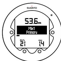
4. Adjust the PO<sub>2</sub> (oxygen partial pressure) value with [DOWN] or [UP] and accept with [SELECT].
