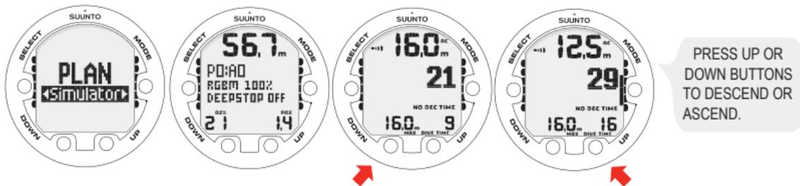
The mode can also be used to add the desired surface intervals for dive simulations. Add the desired surface interval increments to the present surface interval by pressing the UP and DOWN buttons.
