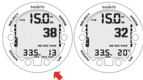
UP BUTTON TOGGLES BETWEEN DIVE TIME AND WATER TEMPERATURE.
