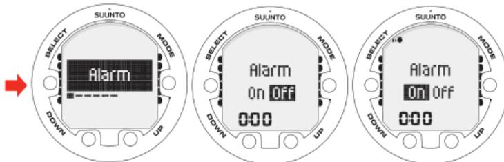
ADJUST WITH UP AND DOWN BUTTONS. ACCEPT WITH SELECT BUTTON.
