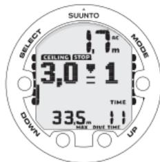
WHEN CEILING AND STOP ARE DISPLAYED, IMMEDIATELY (WITHIN 3 MINUTES) DESCEND TO OR BELOW CEILING.
