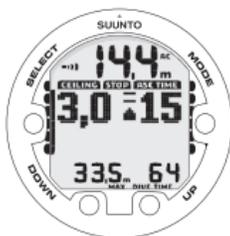
UPWARD POINTING ARROW, BLINKING ASC TIME AND AN ALARM TELL YOU TO ASCEND. MINIMUM TOTAL ASCENT TIME INCLUDING MANDATORY SAFETY STOP IS 15 MINUTES. CEILING IS AT 3 M.
