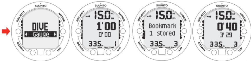
BY PRESSING THE SELECT BUTTON DURING A DIVE, A BOOKMARK IS WRITTEN IN THE PROFILE MEMORY, THE DIVE TIMER IS RESET, AND THE PREVIOUSLY-TIMED INTERVAL IS DISPLAYED BELOW.
