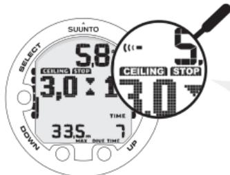
WHEN CEILING AND STOP ARE DISPLAYED, MAKE A ONE MINUTE MANDATORY SAFETY STOP IN THE DEPTH ZONE BETWEEN 6 M AND 3 M.
