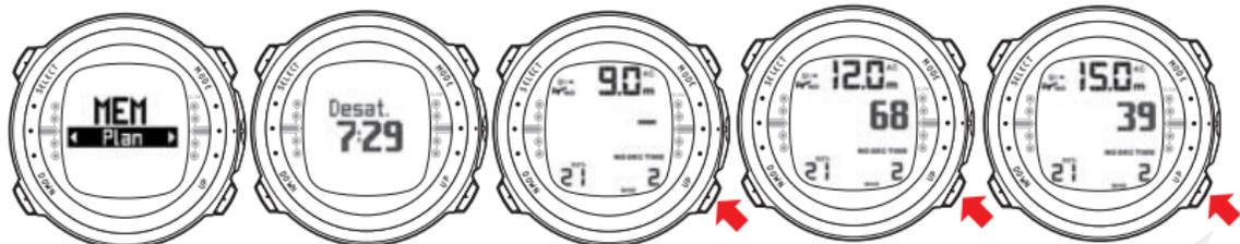
QUANDO SI ATTIVA LA MODALITÀ MEMPLAN, IL DISPLAY MOSTRA BREVEMENTE IL TEMPO DI DESATURAZIONE RIMANENTE PRIMA DI PASSARE ALLA MODALITÀ PLAN. PREMERE I PULSANTI UP E DOWN PER SCORRERE TRA I DIVERSI LIMITI DI NON DECONPRESSIONE. I LIMITI DI NON DECONPRESSIONE SUPERIORI A 99 MINUTI SONO VISUALIZZATI CON IL SIMBOLO “—”.
