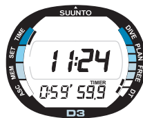
Fig. 2.9. The Downtimer counts down from a pre-set time and the DT mode indicator flashes.
