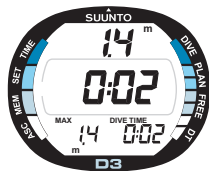
Fig. 3.11. Freedive. Present depth is 1.4m and dive time is 2 seconds.
