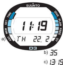
Fig. 2.5. The timekeeping display a) the date is displayed b) the seconds are displayed
