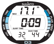
Fig. 3.21. Surface display. You have surfaced from a 44 minute dive, which had a maximum depth of 17.1m [ft].
