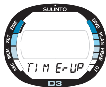
Fig. 2.6. The Stopwatch function is indicated by the TIMER UP text and a mode indicator.
