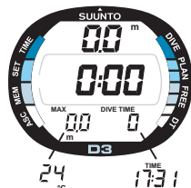
Fig. 3.5. Startup III. Surface Mode (Gauge). Depth and dive time are zero. Pressing +/- button activates alternate display of maximum depth and current time.
