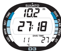
Fig. 3.18. Diving display. Present depth is 10.2m. Dive timer shows 27 minutes and 18 seconds. Temperature and dive time are shown in the bottom window.
