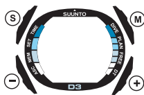
Fig. 2.1. The push buttons of the D3.
