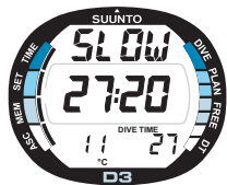
Fig. 3.20. Ascent Rate Indicator. Blinking SLOW and four segments are shown together with an audible alarm. Ascent Rate is more than 10 m/min [33ft/min].
