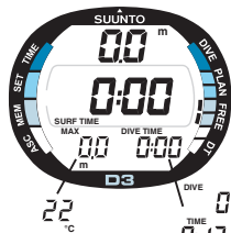
Fig. 3.6. Startup IV. Free mode. Depth and dive time are zero. Pressing +/- button activates alternate displays.
