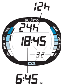
Fig. 4.3. The Time Adjustment Mode is activated and the second digits are blinking. Page I.
