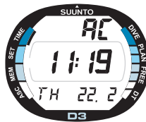
Fig. 2.3. Active water contact is indicated by the text AC.
