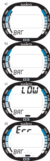
Fig. 3.4. Startup II. Battery Power Indicator.
