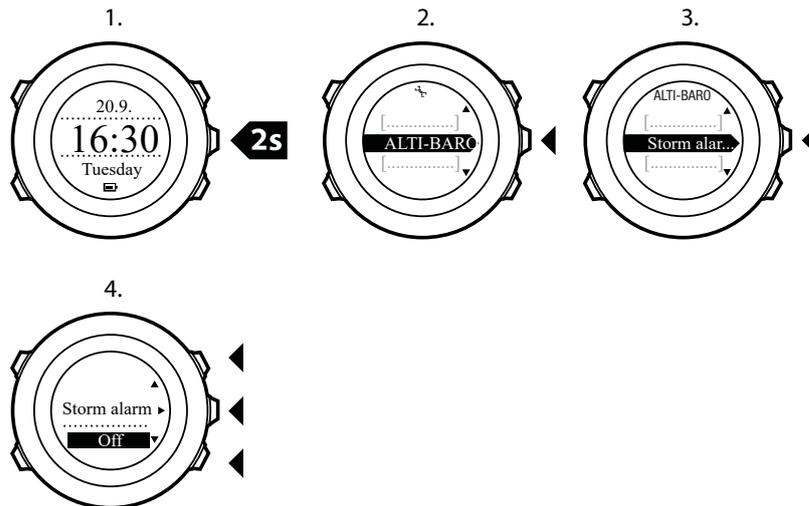
When a storm alarm occurs, pressing any button ends the alarm. If no button is pressed, the alarm repeats once after five minutes. The storm symbol remains on the display until the weather conditions stabilize (pressure drop slows down).
