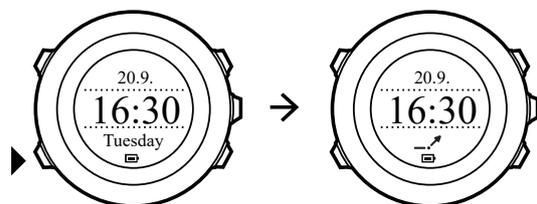
The weather trend indicator is comprised of two lines forming an arrow. Each line represents a 3-hour period. A change in barometric pressure greater than 2 hPa / 0.59 inHg over three hours triggers a change the direction of the arrow. For example:
