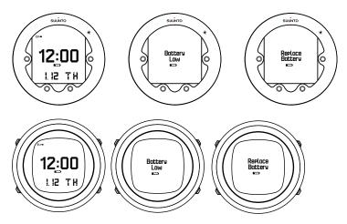
If the low battery icon appears in surface mode, or if the display looks faded, the battery may be too low. Battery replacement is recommended.
