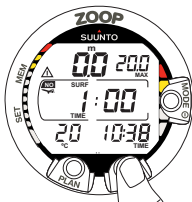
Fig. 3.27. Surface interval, Surface time display. Pressing TIME button once will show surface time display.
