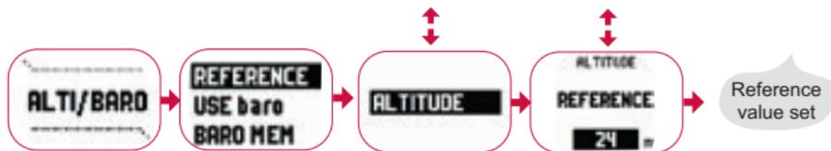
**NOTE:** When the GPS is on, find the altitude reference from the position display in the Function menu.
