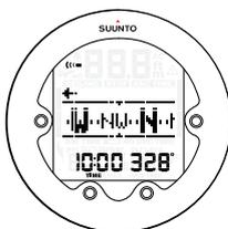
2. Press [MODE] to exit the compass display. If you are underwater, keep [SELECT] pressed to exit.
