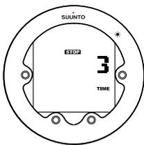
**📄 NOTE:** *When deepstops are enabled, the length of mandatory safety stops is indicated in seconds.*
