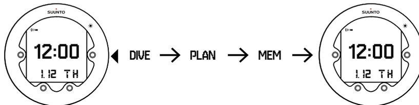
Time and dive modes have different views in the bottom row which you can scroll through with [DOWN] and [UP].
