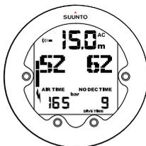
The change in your air consumption is based on constant one second interval pressure measurements over periods of 30–60 seconds. An increase in air consumption decreases the remaining air time rapidly, while a drop in air consumption increases the air time slowly. In this way, an overly optimistic air time estimate, caused by a temporary drop in air consumption, is avoided.
