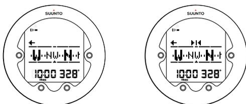
If, at any point, your bearing moves outside the compass display, right or left arrows appear to show turn direction.
