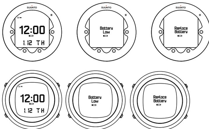
If the low battery icon appears in surface mode, or if the display looks faded, the battery may be too low. Battery replacement is recommended.
