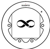
Calibrate the compass by slowly rotating the unit in your hand in large figure-8 loops..
