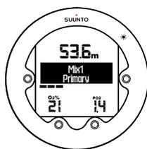
5. Adjust the blinking O<sub>2</sub> value with [DOWN] or [UP] to match the oxygen % of your tank and accept with [SELECT] .
