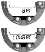
Figur 5.6. Start II. Batteriindikator.
