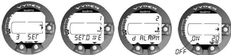
Figure 5.2. Setting Dive Time Alarm. Press scroll buttons to change alarm on/off and to set dive time value.
