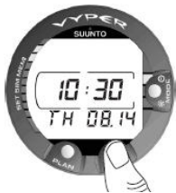
Figure 3.1. Time keeping display. Press the PLAN or TIME button to activate the display.
