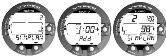
Figure 7.13. Dive Planning Simulator mode [2 SIMPLAN]. Add desired surface interval increment (to present shown surface interval) by pressing TIME and PLAN buttons. This display is only shown for repetitive dives.
