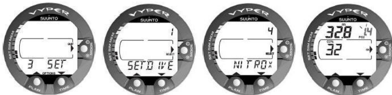
Figure 5.4. Setting Oxygen Percentage and Partial Pressure. The equivalent maximum depth is displayed as 32.8 m / 107 ft. Press scroll buttons to change oxygen percentage and to set oxygen partial setting value.
