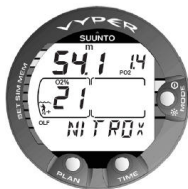
Figure 6.11. Nitrox display. Maximum depth based on set O_2\% (21%) and PO_2 (1.4 bar) is 54.1 m/177 ft.
