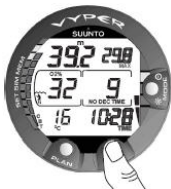
Figure 6.13. Alternative display. Pressing the TIME button displays the current time, maximum depth and CBT.
