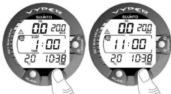
Figure 7.2. Surface interval, the surface time and no-flying time displays: Pressing the TIME button once the surface time display is shown and by pressing the TIME button twice the no-flying time display is shown, indicated by the airplane symbol.
