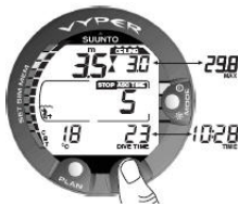
Figure 6.9. Decompression dive, at ceiling zone. Two arrows point at each other (“hour glass”). You are in the optimum ceiling zone at 3.5 m/11 ft and your minimum ascent time is 5 minutes. Pressing TIME button activates alternative display.
