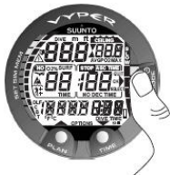
Figure 5.5. Startup I. All segments shown.
