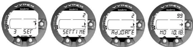
Figure 4.6. Adjusting the Date setting mode [2 Adj DATE].
