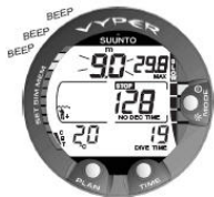
Figure 6.4. Ascent Rate Indicator. Blinking depth reading, SLOW and four segments shown: ascent rate is more than 10 m/min/33 ft/min. This is a caution to slow down! The STOP sign means that you are advised to make a Mandatory Safety Stop when you reach the depth of 6 m/20 ft.
