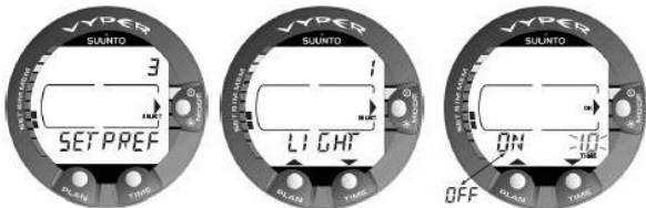
Figure 4.8. Setting Backlight On Time. Press scroll buttons to change backlight on/off and to set time value.
