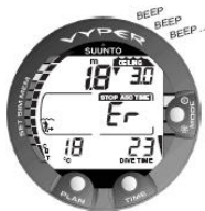
Figure 6.10. Decompression dive, above ceiling. Note a downward pointing arrow, an Er warning and an audible alarm. You should immediately (within 3 minutes) descend to or below ceiling.
