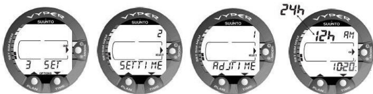
Figure 4.5. Adjusting the Time setting.
