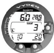
Figure 5.8. Ascent rate indicator. Two segments.
