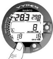
Figure 6.3. Diving display. An annotation, Bookmark, is done in the profile memory during a dive by pressing the PLAN button. Note the Logbook symbol.
