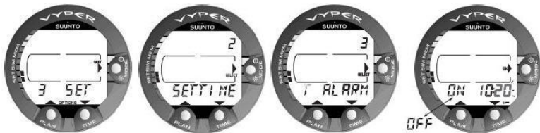
Figure 4.7. Adjusting the Daily Alarm setting mode [3 T ALARM]
