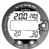
Figure 6.15. The Gauge mode. The present depth, maximum depth, dive time, remaining air time and ascent rate indicator are displayed during the dive.
