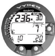
Figure 6.7. Decompression dive, below floor. Upward pointing arrow, blinking ASC TIME label and an audible alarm tell you to ascend. Minimum total ascent time including safety stop is 7 minutes. Ceiling is at 3 m/10 ft.
