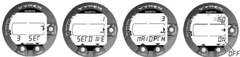
Figure 5.3. Setting Maximum Depth Alarm. Press scroll buttons to change alarm on/off and to set maximum depth value.
