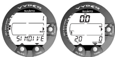
Figure 7.12. Dive Simulator mode [1 SIMDIVE]. Descend by pressing the arrow down (TIME) button and ascend by pressing the arrow up (PLAN) button.
