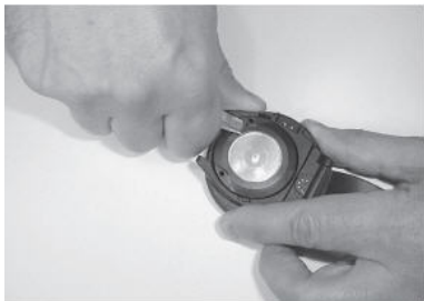
Figure 9.1. Opening of the securing ring.
