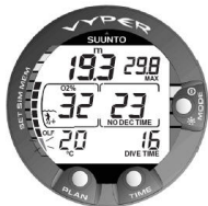
Figure 6.14. The lowest bar graph blinks to indicate that the OLF value shown relates to OTU.
