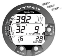
Figure 6.12. Oxygen partial pressure and OLF displays. There is an audible alarm as oxygen partial pressure is greater than 1.4 bar or set value, and/or the OLF has reached 80% limit.
