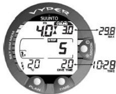
Figure 5.9. A Mandatory Safety Stop. You are advised to make a Mandatory Safety Stop in the depth zone between 6 m and 3 m/20 ft and 10 ft. Press the TIME button to view the alternative display.
