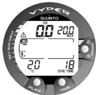
Figure 7.1. Surface display. You have surfaced from a 18 minute dive, which maximum depth was 20.0 m/66 ft. The present depth is 0.0 m/0 ft. The Airplane symbol indicates that you should not fly and diver attention symbol indicates that you should prolong your surface interval time.
