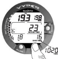
Figure 6.2. Diving display. Present depth is 19.3 m /63 ft and nodecompression stop time limit is 23 minutes in A0/P1 mode. Maximum depth during this dive was 19.8 m/65 ft, elapsed dive time is 16 minutes. The current time 10:20 [10:20 am] is shown for 5 seconds after pressing the TIME button.
