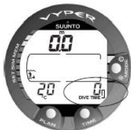
Figure 5.7. Low Battery Warning. Battery symbol indicates that the battery is low and battery replacement is recommended.
