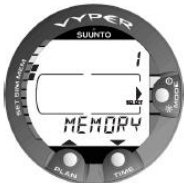
Figure 4.2. Scroll the mode options by pressing the arrow up/ down buttons.
