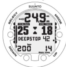
DURANTE LA RISALITA VIENE VISUALIZZATA LA NECESSITÀ DI EFFETTUARE UNA SOSTA DI PROFONDITÀ A 25 METRI PER LA DURATA INDICATA DAL TIMER (42 SEC. RIMANENTI).
