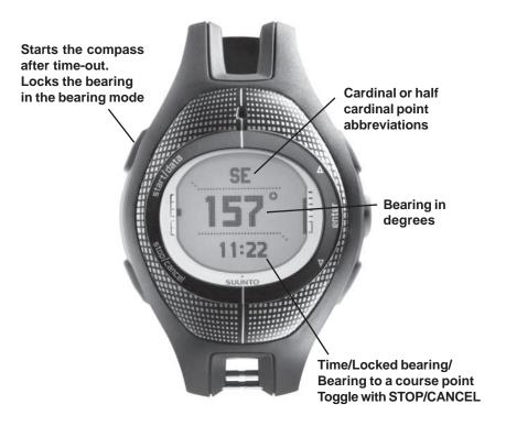
The Compass mode utilizes the Suunto 9-series 3D compass, which allows reading the compass reliably even if the unit is held tilted up to 30 degrees from horizontal to any direction.
