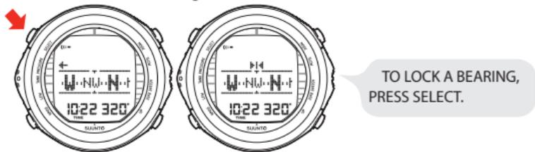
The Suunto D9tx also provides help for navigating square and triangular patterns, as well as navigating a return heading. This is made possible by following graphical symbols in the center of the compass display:
