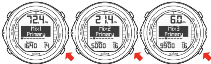
When in the MIXED setting mode, the equivalent maximum operating depth, based on the chosen setting, is also displayed.
