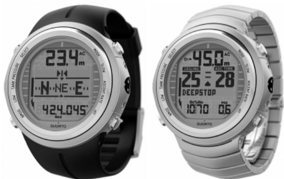
Suunto D9tx is the world's first wristop sized dive computer to integrate a tilt-compensated 3D digital compass, wireless tank pressure reception, and trimix functions. It simplifies your diving experience because all the information you need relating to depth, time, optional tank pressure, decompression status, and direction is now available on one easy-to-read screen.
