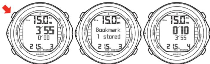
BY PRESSING THE SELECT BUTTON DURING A DIVE, A BOOKMARK IS WRITTEN IN THE PROFILE MEMORY, THE DIVE TIMER IS RESET, AND THE PREVIOUSLY-TIMED INTERVAL IS DISPLAYED BELOW.
