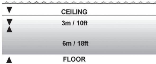
The depth of the ceiling and floor depends on your dive profile. The ceiling depth will be fairly shallow when you enter the decompression mode, but if you remain at depth, it will move downward and the ascent time will increase. Likewise, the floor and ceiling may change upwards while you are decompressing.
