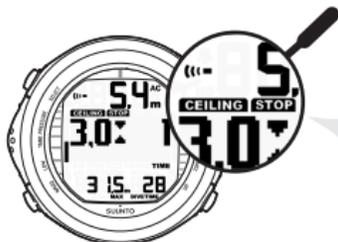
WHEN CEILING AND STOP ARE DISPLAYED, MAKE A ONE MINUTE MANDATORY SAFETY STOP IN THE DEPTH ZONE BETWEEN 6 M AND 3 M.
