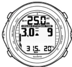
UPWARD POINTING ARROW, BLINKING ASC TIME AND AN ALARM TELL YOU TO ASCEND. MINIMUM TOTAL ASCENT TIME INCLUDING SAFETY STOP IS 9 MINUTES. CEILING IS AT 3 M.
