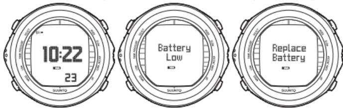
If the battery symbol is displayed in the Surface mode, or if the display is faded or weak, the battery may be too low to operate the dive computer, and battery replacement is recommended.
