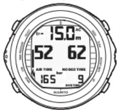
CURRENT TANK PRESSURE IS 165 BAR AND THE REMAINING AIR TIME IS 52 MINUTES.
