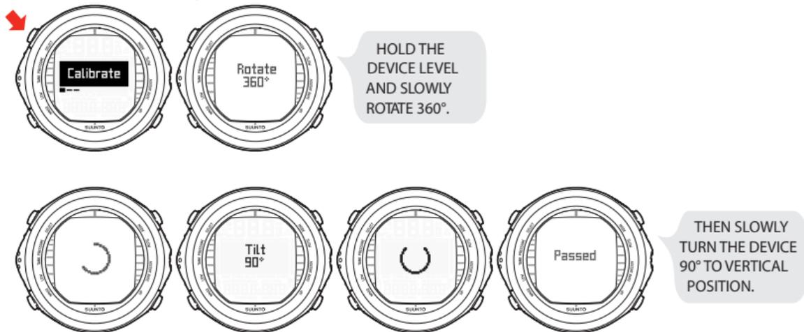
If the calibration fails several times in a row, it is possible that you are in an area with sources of magnetism, such as large metal objects, power lines or electric appliances. Move to another location and try to calibrate the compass again. If the calibration continues to fail, contact an authorized Suunto service center.
