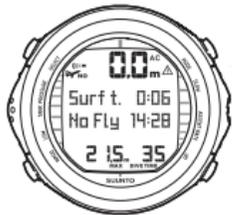
IT IS 6 MINUTES SINCE YOU SURFACED FROM A 35-MINUTE DIVE. THE MAXIMUM DEPTH WAS 21.5 M. THE PRESENT DEPTH IS 0.0 M. THE AIRPLANE SYMBOL AND NO-FLY VALUE INDICATE THAT YOU SHOULD NOT FLY FOR 14 HOURS, 28 MINUTES. THE DIVER ATTENTION SYMBOL INDICATES THAT YOU SHOULD PROLONG YOUR SURFACE INTERVAL TIME.
