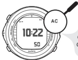
AC APPEARS IN THE TOP RIGHT CORNER OF THE DISPLAY, WHEN THE DIVE COMPUTER IS IN CONTACT WITH WATER. THIS ALSO ACTIVATES THE DIVE MODE.
