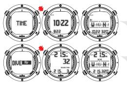
IF ACCESSED FROM TIME MODE, TIME AND BEARING ARE DISPLAYED AT THE BOTTOM OF THE SCREEN.
